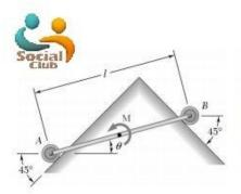
Uniform rod AB of length l and weight W lies in a vertical plane and is acted upon by a couple M. The ends of the rod are connected to small rollers which rest against frictionless surfaces. (a) Express the angle  $\theta$  corresponding to equilibrium in terms of M, W, and l. (b) Determine the value of  $\theta$  corresponding to equilibrium when  $M = 1.5 \text{ lb} \cdot \text{ft}$ , W = 4 lb, and l = 2 ft.
