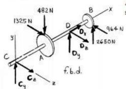
Assume moment reactions at the bearing supports are zero. From f.b.d. of shaft
