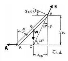
(a) As shown in the f.b.d. of the slender rod AB, the three forces intersect at C. From the geometry of the forces
