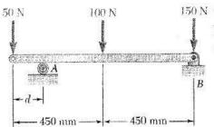
150 N The maximum allowable value of each of the reactions is 180 N. Neglecting the weight of the beam, determine the range of the distance d for which the beam is safe.
