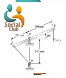
A lever AB is hinged at C and is attached to a control cable at A. If the lever is subjected to a 300-N vertical force at B, determine (a) the tension in the cable, (b) the reaction at C.
