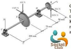
Gears A and B are attached to a shaft supported by bearings at C and D. The diameters of gears A and B are 150 mm and 75 mm, respectively, and the tangential and radial forces acting on the gears are as shown. Knowing that the system rotates at a constant rate, determine the reactions at C and D. Assume that the bearing at C does not exert any axial force, and neglect the weights of the gears and the shaft.
